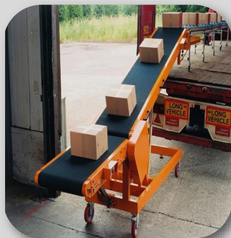
TRUCK LOADING CONVEYOR
